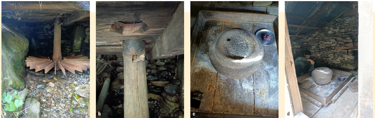
Figure 9 Characteristics of choskor (watermill) of Dikshipam village. (a). Wooden propeller/turbine (chhoskor-yapche), (b). Wooden adjuster (sarr) attached to the vertical wooden pole (zung-seng), (c). Chhoskor attached to propeller, while resting on a wooden plank (bleng), (d). Measuring the mean size of the chhoskor (Dikshipam village). Source: Thongdok and Sati 2024
