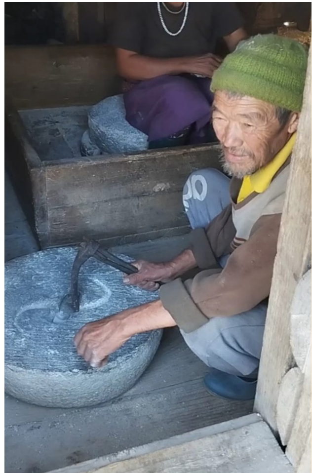
Figure 3 Zyopo (craftsperson) manufacturing grinding stones for watermill
